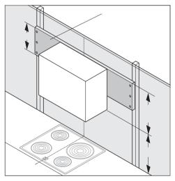
Determine and mark the top edge of the appliance. It must be at least S + 17 <sup>3</sup>/<sub>4</sub>" (S + 450 mm) in order to comply with the safety height (see "Appliance Dimensions").
